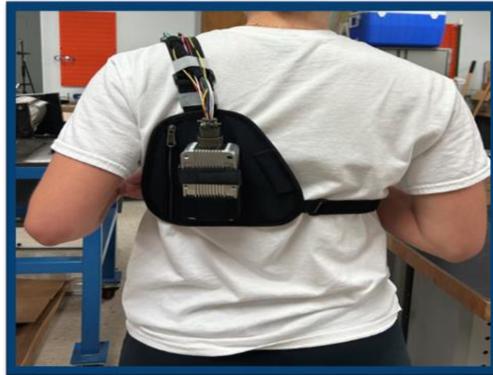
The modular gas box would be placed inside the straps on the back of the mount
